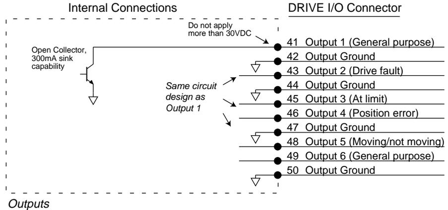
You can use the OUTLVL command to configure each of the outputs as active high or active low.
